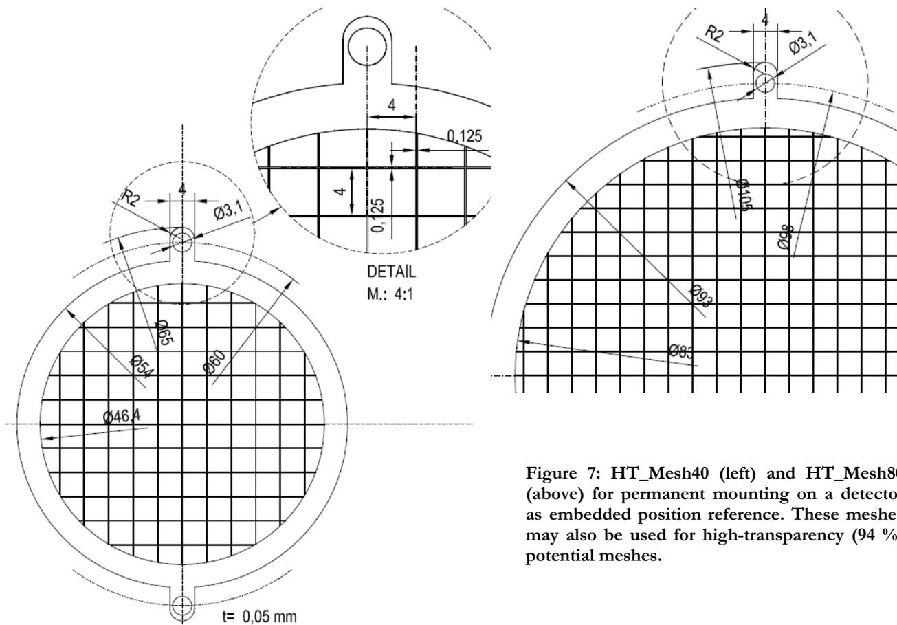
Figure 7: HT\_Mesh40 (left) and HT\_Mesh80 (above) for permanent mounting on a detector as embedded position reference. These meshes may also be used for high-transparency (94 %) potential meshes.
