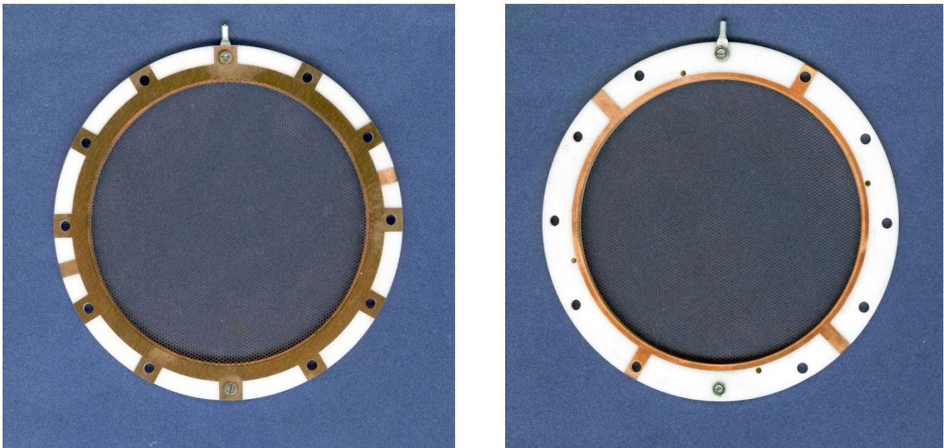
Figure 3: Free-standing Mesh80 mounted to the MCP front ring (left: front side, right rear side of the front ring).
