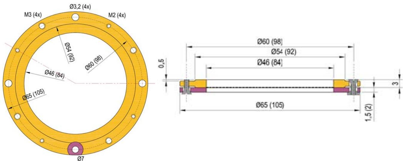
Figure 2: Sketch of wMesh40/80 (displayed here: wMesh40) showing all dimensions (for Mesh80 in parentheses if different). The **RoentDek** meshes can be mounted right onto the front ceramic ring (wMesh120: via spacers).
