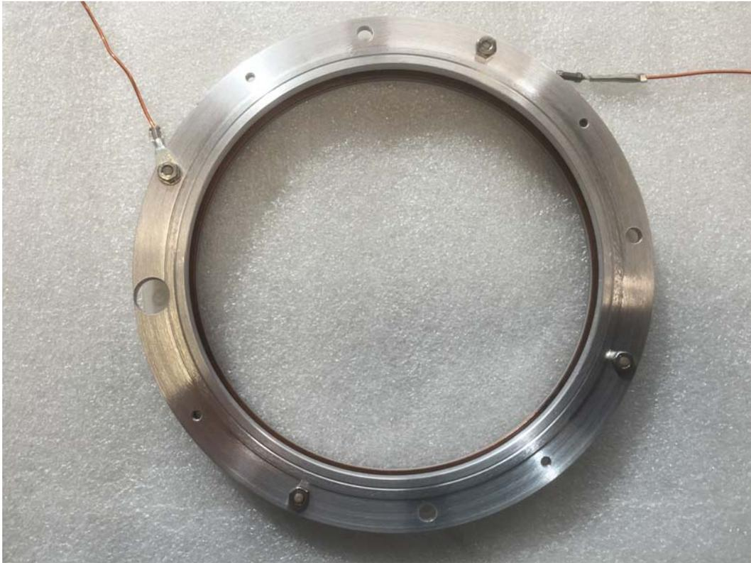
**Figure 9: wMesh80 mounted on ceramic ring with contact cable for mesh bias.**
