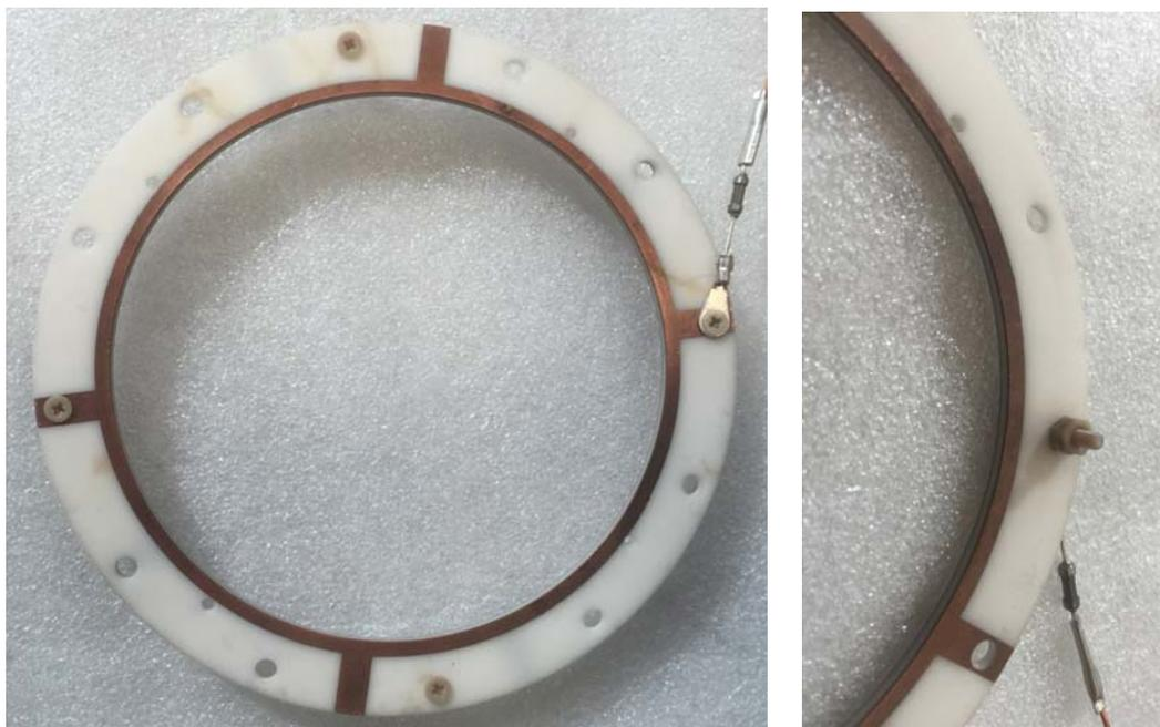
Figure 8: MCP front clamping ring with bias contact, here for Hex80/DLD80 (left: side facing towards MCP, right: other side). Thermoplastic screws are used to enhance high voltage withstanding.
