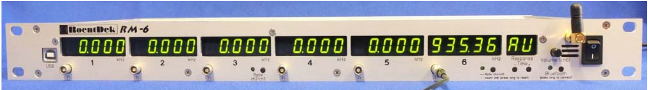
Figure 1: RM-6 counter module. Several displays allow simultaneous observation of up to six count rates.
