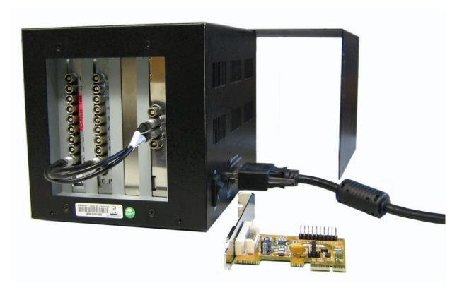
PCI2PCIe crate, here with two TDC8HP boards and clock card inserted for synchronization. A PCIe adapter card and cable connection is shown on the lower right side. Not shown is the mains adapter (12V, 3A) with cable.
